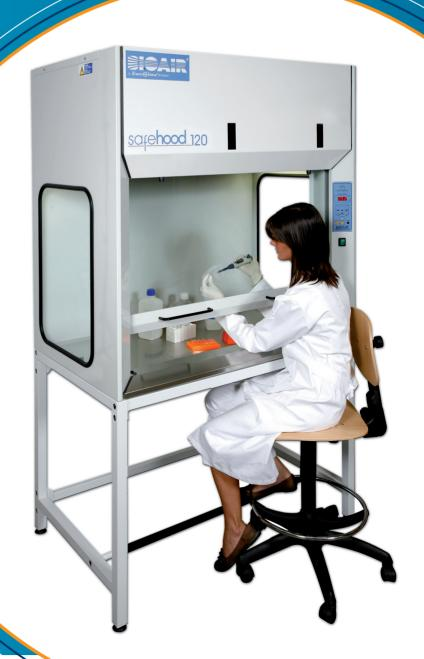
Safehood is the new Bioair fume cupboard with activated carbon filters for the removal of toxic fumes, gases or vapours from the exhausted air.
