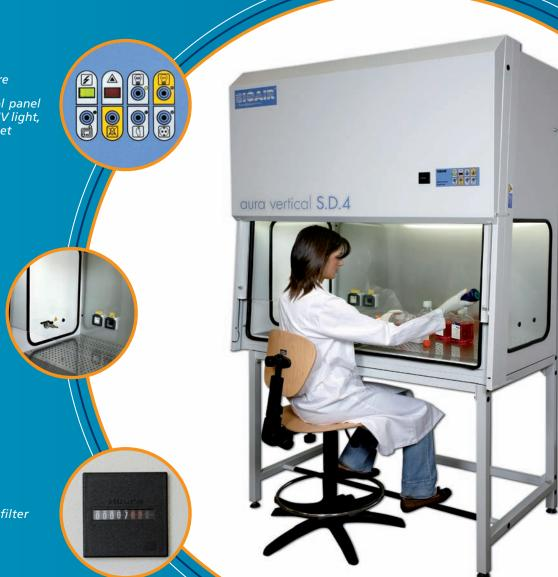
Aura Vertical S.D.4 is a partial-recirculating Class 100 vertical laminar airflow: air coming through the front aperture is mixed underneath the work surface with the downflow air and recirculated.
